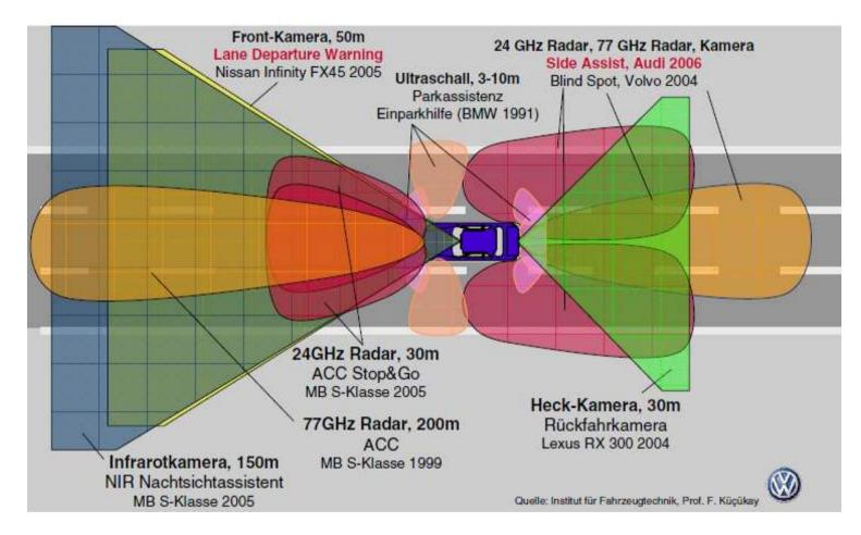
Ü Different types of sensors for measuring the environment
