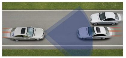
Unavoidable collision with oncoming traffic Activation of the PRE-SAFE<sup>®</sup> belt tensioners based on information from the close-range radar
