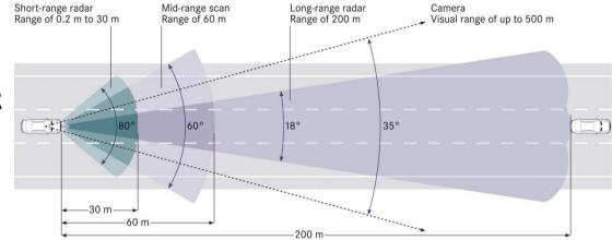
Frequency-Modulated-Continous-Wave priciple (FMCW), two microprocessors, Field-Programmable-Gate-Array
