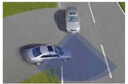
Unavoidable collision at a junction Activation of the PRE-SAFE® belt tensioners based on information from the close-range radar
